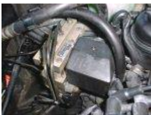
Figure 6 Typical ABS ECU located in the engine bay.
