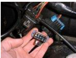
Figure 5 The ALDL is a 10-pin connector.
