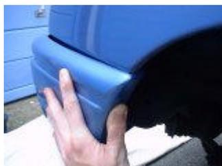
Once the hole is drilled, put some rust stopper on the fresh
