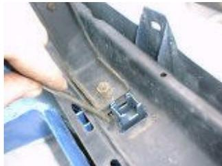
With the bumper off, remove the carriage bar from the back. This is tricky, squash each plastic clip and pull the carriage bar off (may be different on some types of bumper).
