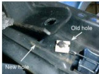
The new MK2 irons do not bolt in the same place as the MK1 irons. Fortunately there is a hole for the MK2 irons to fit on the MK1 carriage bar already.
