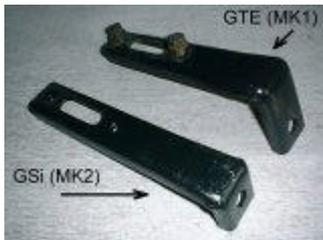
However, you need to acquire the longer Nova GSi irons (2 off). Otherwise the bumper will not fit on the car (holes do not line up).
