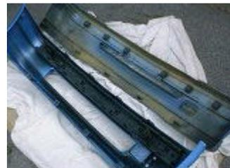
Pop the carriage bar, with the MK2 irons in place, onto the back of the GSi front bumper (it snaps into place).
