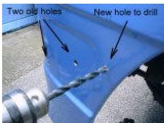
A new hole needs to be drilled on each wing where the bolt that
