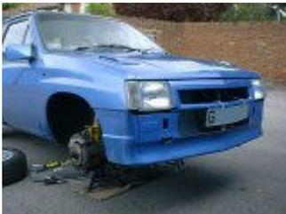
Jack up the car and remove the front bumper (2 bolts under each arch, 4 bolts for each side wing). Follow the Haynes book for details.
